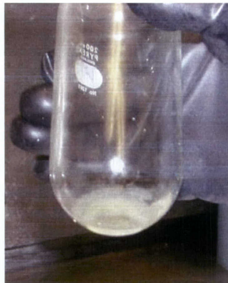
Photo 2.2 Gelled Residue Found in the Bottom of the Liquid GB Sample Container
